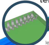
Our patented design weaves the antenna through the circuit board 20 times per centimetre, and much like a coiled spring the effective length of the antenna is 5 times the physical length it consumes. It's like having a 75cm long antenna in a single 15cm sensor. A larger antenna increases the resolution and sample area of each sample, allowing more noise to be filtered out. This gives highly accurate tracking of moisture changes with no "dead spots".
